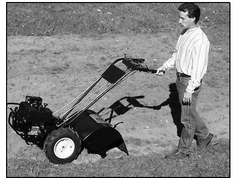
Figure 4-2: Use one hand to guide tiller when moving forward.
